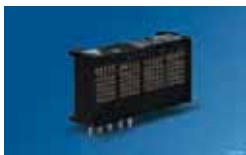
SCDQ554XQ Display Serial Input with a Character RAM SIP Package Pinout with 90 Degree Formed Leads Page / Seite: 99
